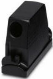
HEAVYCON ADVANCE for increased environmental requirements, sleeve housing B16, with bayonet locking, height 100 mm, with 1xM40 thread, lateral cable outlet
