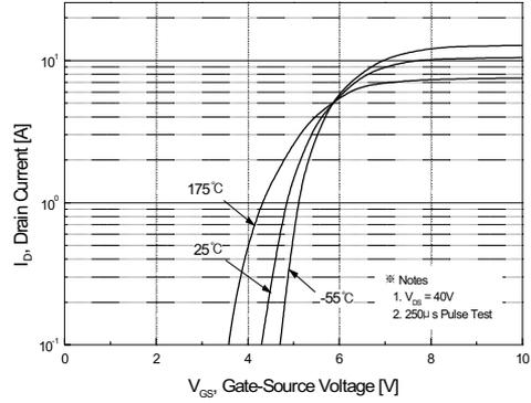
Figure 2. Transfer Characteristics
