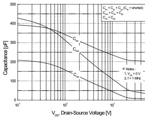
Figure 5. Capacitance Characteristics
