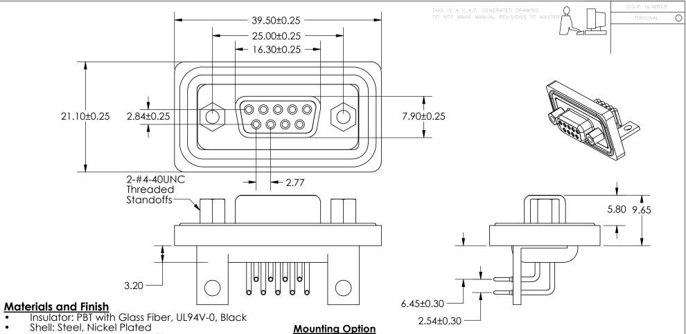
Contact: Copper Alloy, with 2-Gold Flash Plating over Nickel Watertight Frame: PBT with Glass Fiber, UL94V-0,
