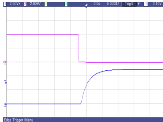
Fig.30 Typical start-up from CNT on of AVQ100B-48S05
