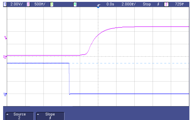
Fig.22 Typical start-up from CNT on of AGQ100-48S1V2
