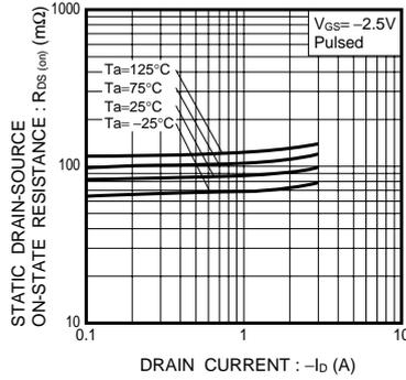
Fig.5 Static Drain-Source On-State Resistance vs. Drain Current
