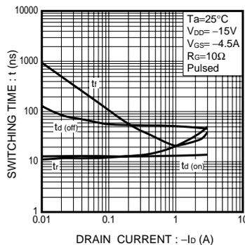
Fig.8 Switching Characteristics
