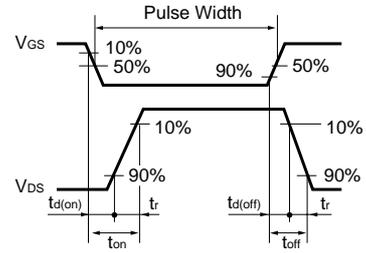
Fig.11 Switching Waveforms
