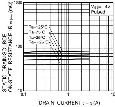
Fig.4 Static Drain-Source On-State Resistance vs. Drain Current
