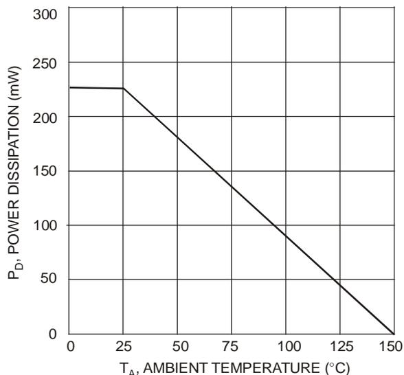
Fig. 1 Power Derating Curve, Total Package (Note 5)
