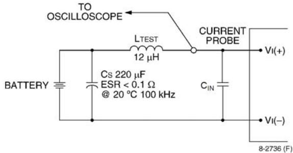
Note: Measure the input reflected-ripple current with a simulated source inductance (LTEST) of 12 μH. Capacitor CS offsets possible battery impedance. Measure the current, as shown above.
