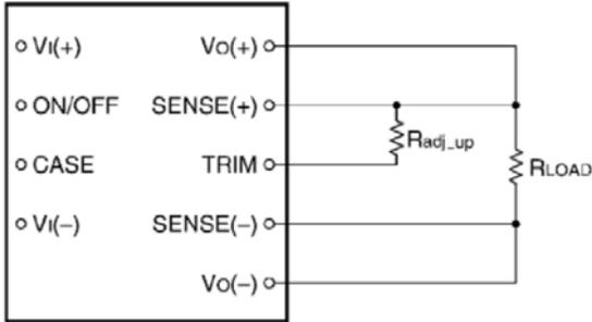
**Figure 14. Circuit Configuration to Increase Output Voltage.**
