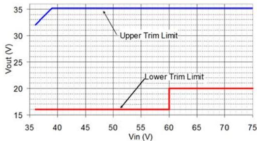
Figure 12. Output Voltage Trim Limits vs. Input Voltage.
