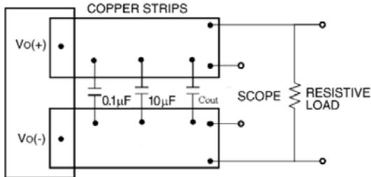
Note: Use a Cout (470 μF Low ESR aluminum or tantalum capacitor typical), a 0.1 μF ceramic capacitor and a 10 μF ceramic capacitor, and Scope measurement should be made using a BNC socket. Position the load between 51 mm and 76 mm (2 in. and 3 in.) from the module.
