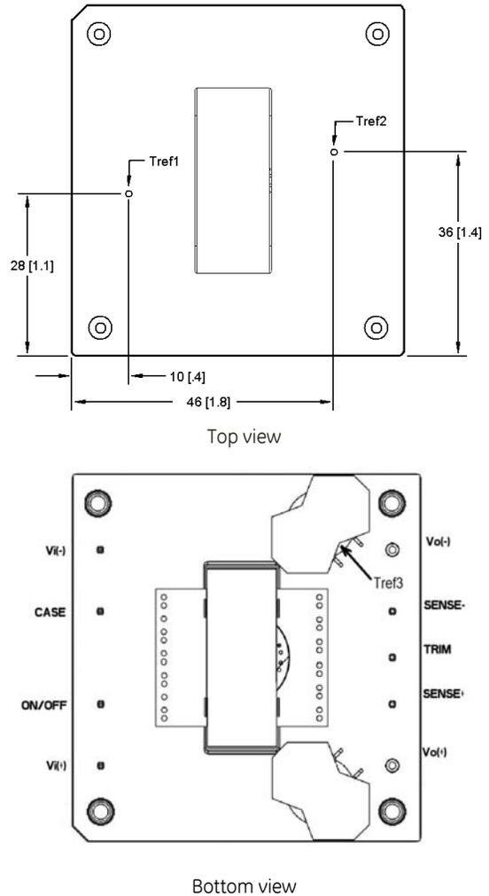
Figure 18. Case ( $T_{REF}$ ) Temperature Measurement Location
