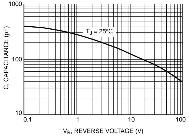
Figure 7. Typical Capacitance
