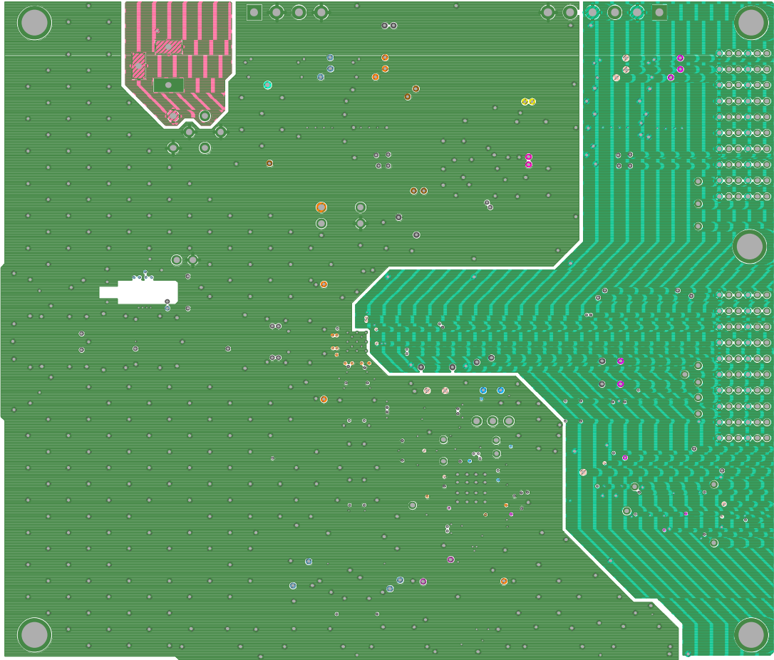
Figure 39. AD9641 Ground Plane (Layer 5)
