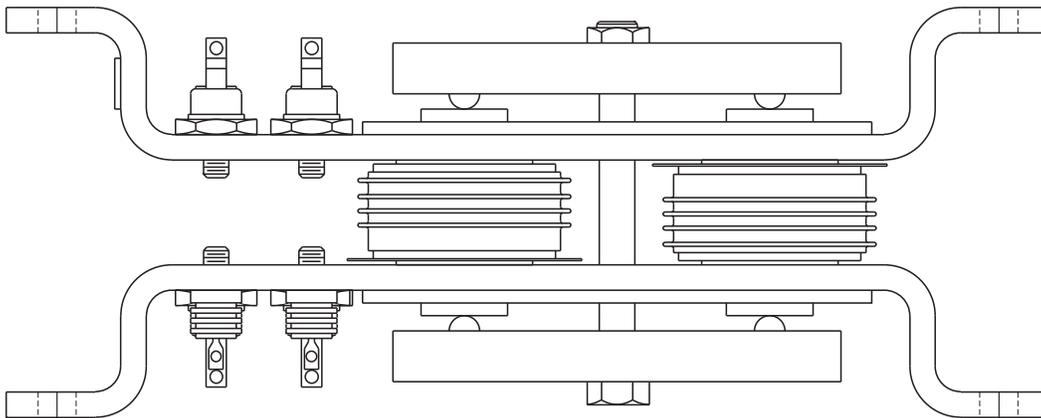
The PPI-600V is a ground-wire device that allows a trailing-cable ground to be monitored independently of the parallel ground path created when trailing-cable-fed equipment is in contact with the earth. It also allows a trailing-cable ground to be monitored in the presence of stray dc and it prevents inter-machine arcing caused by the voltages induced in the cables.
