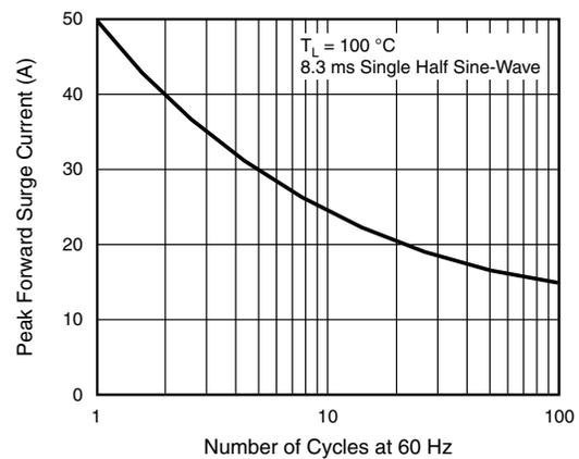
Fig. 2 - Max. Non-Repetitive Peak Forward Surge Current
