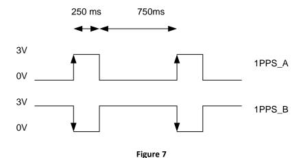
The default pulse width is 250 ms, but is configurable from 100 ms to 500 ms. Typical jitter is 20ns. Signal levels are differential, 0.V to 2.03V.
