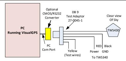
Note: The Yellow test wire are only used when resetting parameters to factory defaults
