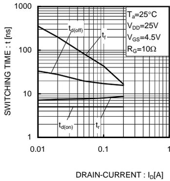
Fig.13 Switching Characteristics
