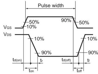
Fig.1-2 Switching waveforms
