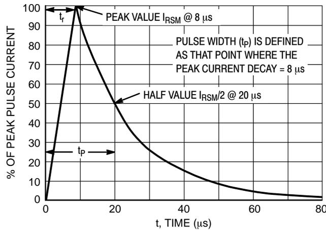
**Figure 1. 8 x 20 μs Pulse Waveform**
