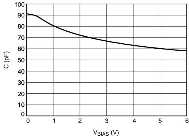
Figure 10. Line Capacitance,  $f = 1$  MHz
