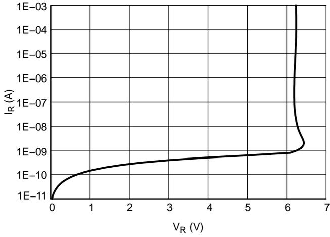
Figure 8. Breakdown Voltage
