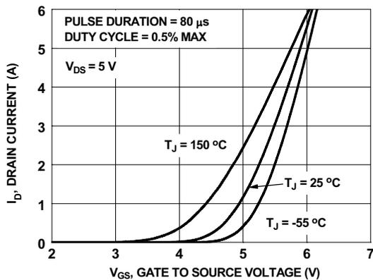
**Figure 5. Transfer Characteristics**
