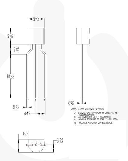
Figure 5. 3Lead, TO-92, MOLDED 0.200 IN LINE SPACING LD FORM (J61Z OPTION)
