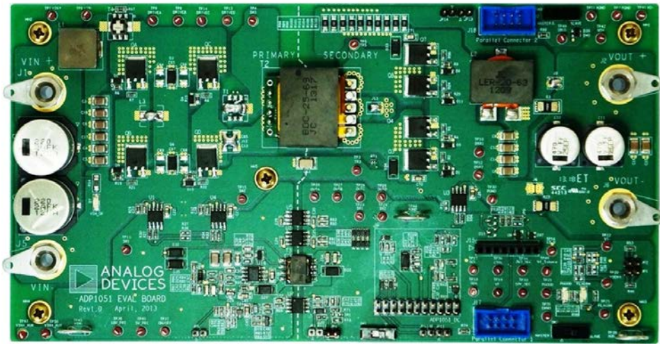
Figure 2. ADP1051-240-EVALZ Evaluation Board
