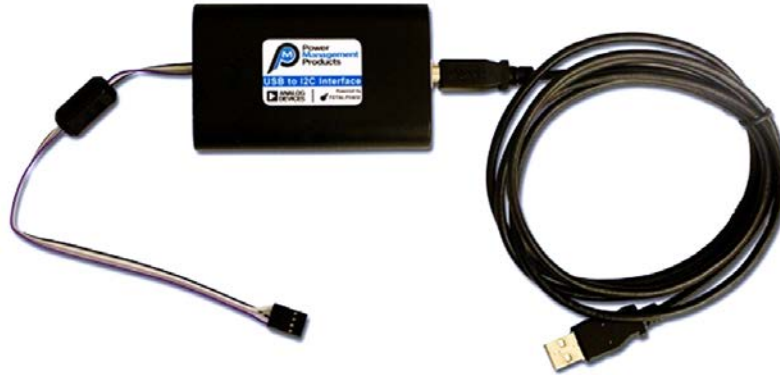
Figure 5. ADP-I2C-USB-Z USB-to-I 2 C Interface Connector
