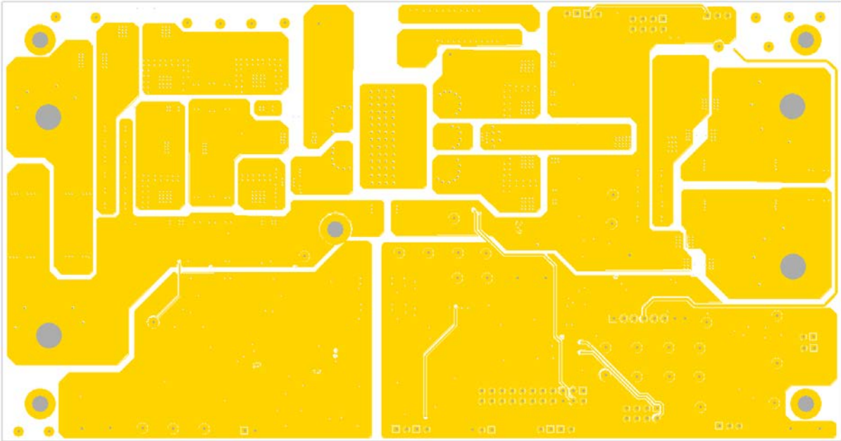
Figure 56. PCB Layout, Bottom Layout
