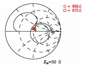
Figure 5: Reflection coefficient at IN port.
