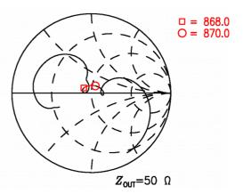
Figure 6: Reflection coefficient at OUT port.
