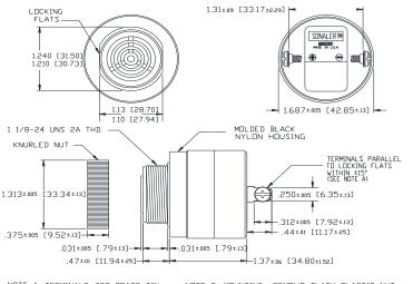
NOTE A: TERMINALS-032 BRASS TIN PLATED, TAPPED FOR #6-32 SCREW. TWO #6-32 NICKEL PLATED BRASS SCREWS INCLUBED. WILL ACCEPT 1/4\* QUICK CONNECT. NOTE B: MOUNTING- REMOVE BLACK PLASTIC NUT AND INSERT THREADED FRINT THROUGH 1.25' HOLE PUNCHED IN PANEL, IF DRIENTATION IS NEEDED, NOTE LOCKING FLATS ON DRAWING. SCREW NUT BACK ON. DO NOT OVERTIGHTEN.
