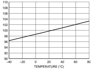
Figure 7. Typical Resistance over Temperature
