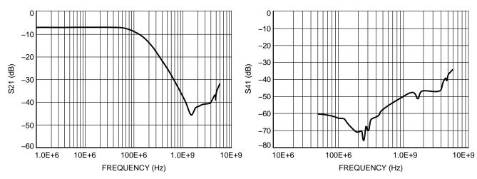
Figure 4. Typical Insertion Loss Curve
