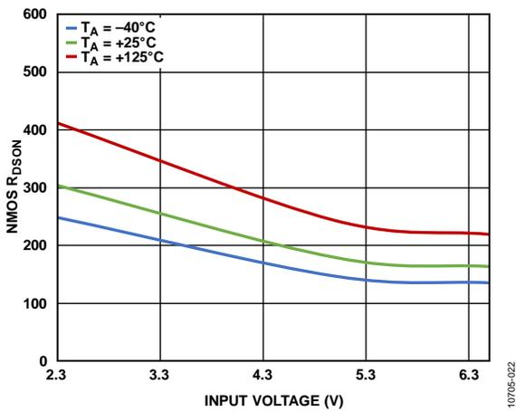
Figure 11. NMOS Drain-to-Source On Resistance ( $R_{DSON}$ )
