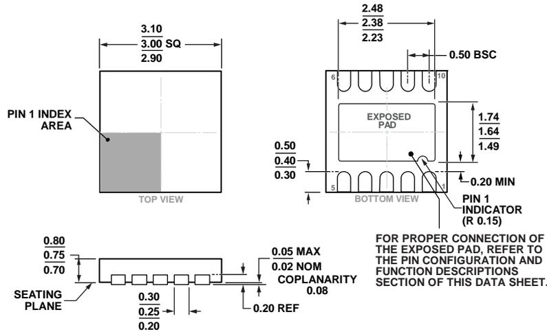
Figure 36. 10-Lead Lead Frame Chip Scale Package [LFCSP\_WD]
