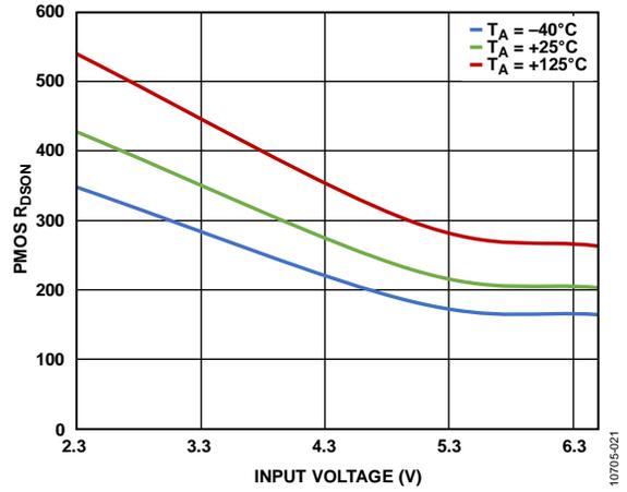
Figure 12. PMOS Drain-to-Source On Resistance ( $R_{DSON}$ )
