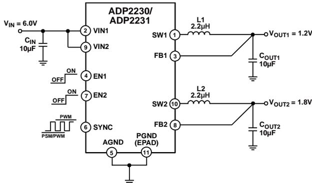
Figure 32. Typical Application Circuit Fixed Output Voltage
