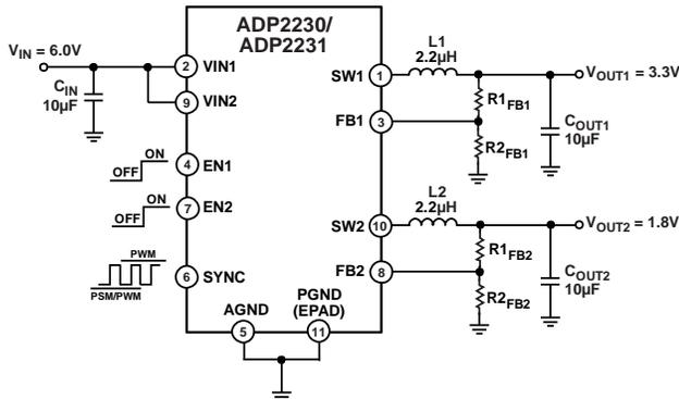
Figure 33. Typical Application Circuit Adjustable Output Voltage
