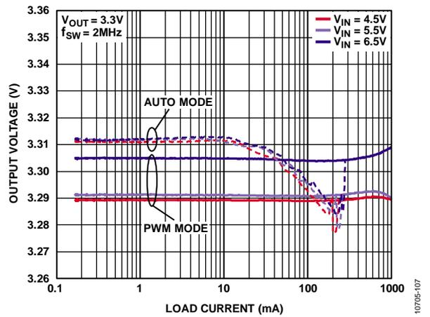
Figure 7. Load Regulation,  $V_{OUT} = 3.3\text{ V}$
