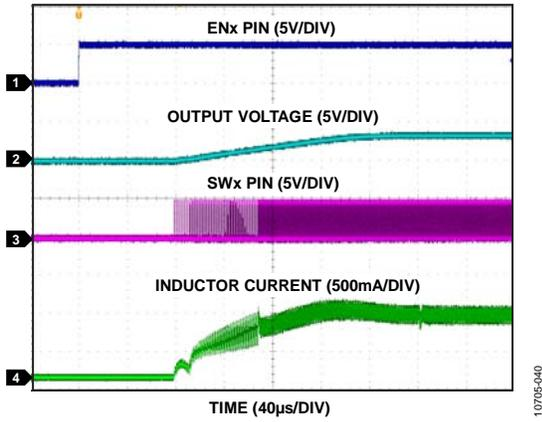
Figure 27. Startup,  $V_{OUT} = 3.3\text{ V}$ ,  $800\text{ mA}$
