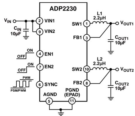
Figure 1. Fixed Output Voltage Typical Application Circuit
