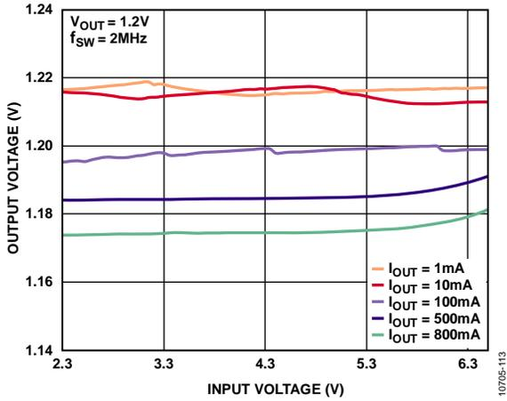
Figure 9. Line Regulation,  $V_{OUT} = 1.2V$ , Different Loads
