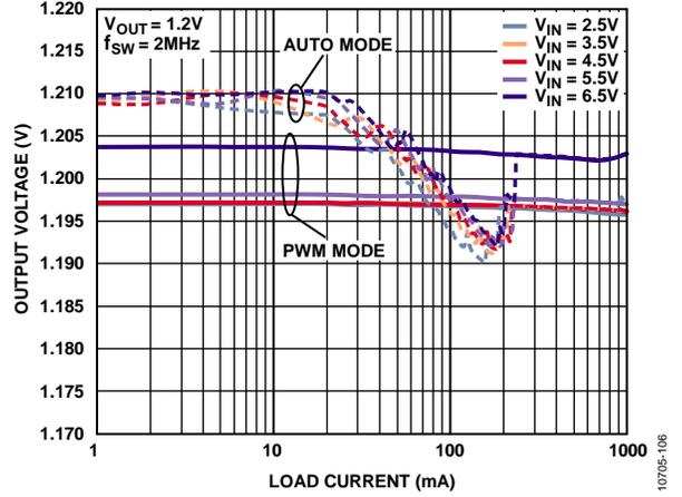
Figure 6. Load Regulation,  $V_{OUT} = 1.2\text{ V}$
