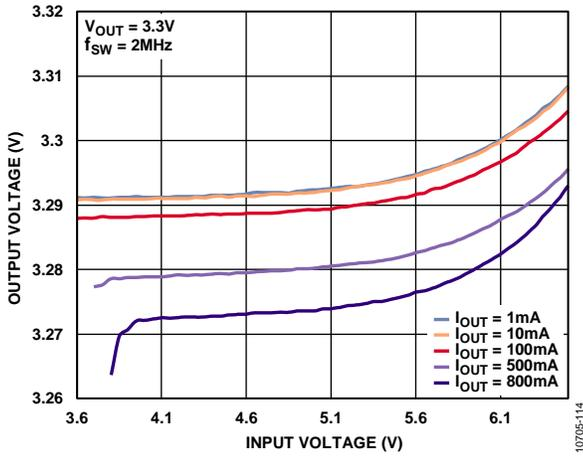
Figure 10. Line Regulation,  $V_{OUT} = 3.3V$ , Different Loads
