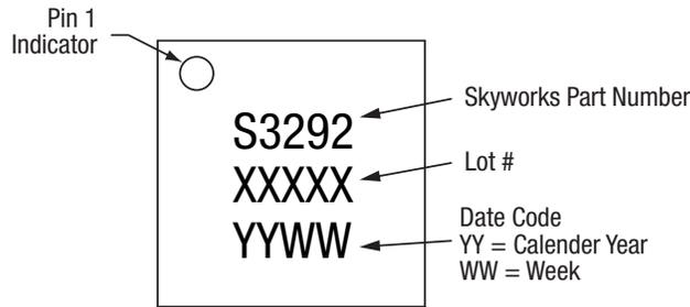
**Figure 13. Typical Case Markings (Top View)**
