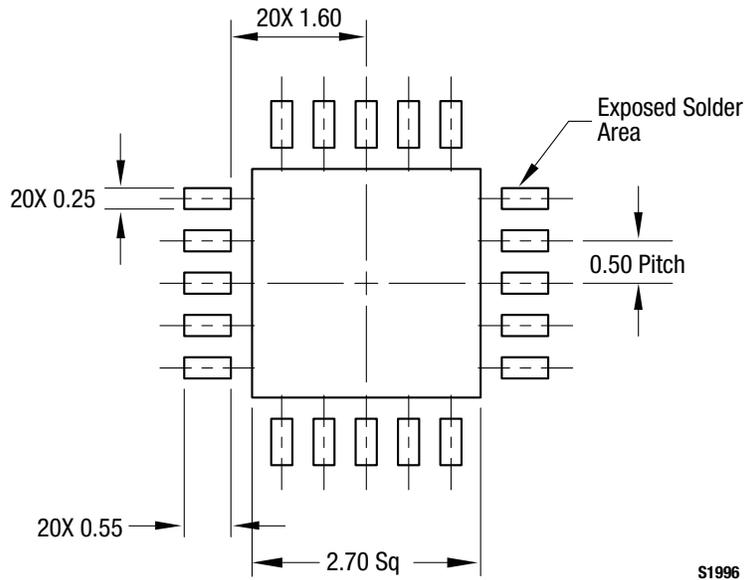
Figure 12. SKY13292-365LF PCB Layout Footprint (Top View)
