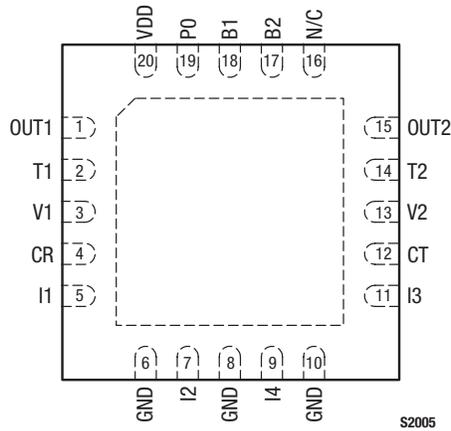
Figure 2. SKY13292-365LF Pinout – 20-Pin QFN (Top View)
