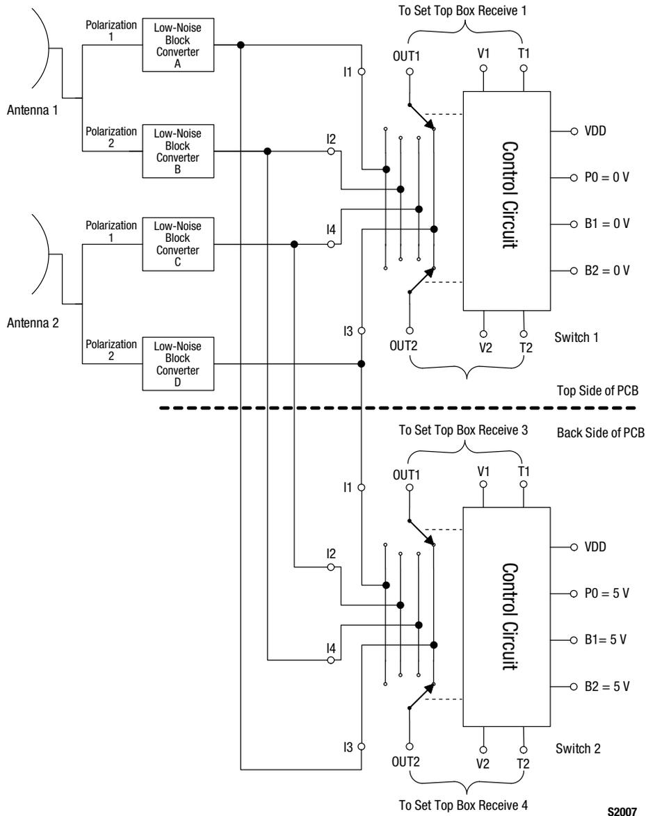
**Figure 3. Suggested Implementation of Two 4x2 Switches**
