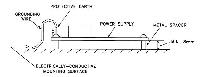
2. TO MEET SAFETY REQUIREMENTS, THE POWER SUPPLY TERMINALS MUST NOT BE USED DIRECTLY AS THE EXTERNAL TERMINATIONS OF ANY EQUIPMENT.
