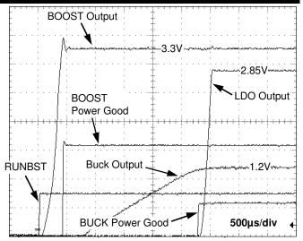
Figure 2. Sequenced Voltages at Start-up
