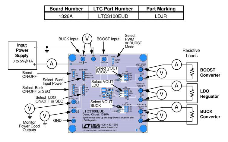
Figure 1. Demonstration Circuit Test Setup
